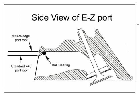
As you can see, by the sectioned port drawing, there is indeed a lip that hangs down from the roof of the intake port on the standard 440 EZ cylinder head. This unique design allows for customers that want to use a standard port intake manifold. We fill in the area behind the lip. Read on to learn more.
