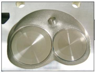
The seat rings are recessed into the casting deep enough to shroud the valves, thereby reducing flow considerably at low and mid-lift openings.
