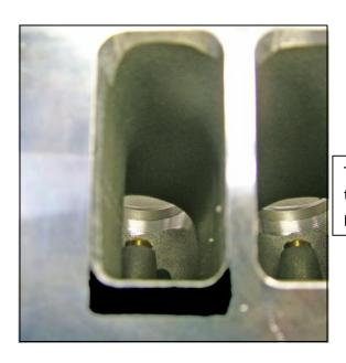
The dark area, shown in the photo to the left, is the lip that is removed to make a Max Wedge size port opening...we can do that if required.
