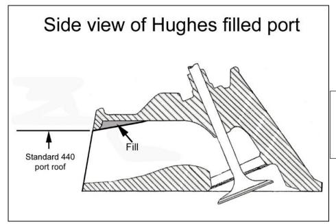
We fill in the area behind the lip as part of our Super Prep and CNC Super prep work. Filling in this area results in a tremendous increase in air flow.
