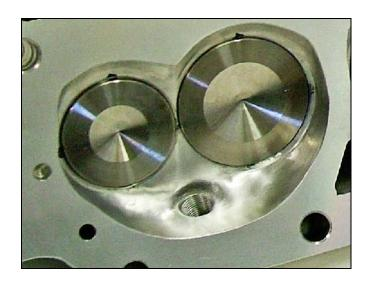
Our C.N.C. machining of the chamber unshrouds the valves and increases the airflow & power output.
