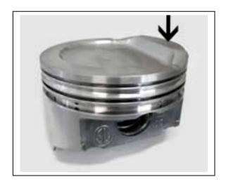
NOTE: When working with a small block stroker kit that is using Keith Black pistons, the top of the small quench dome on the intake side of the piston is where you *MUST* measure the deck from. Normally the point that the arrow is indicating will be .000" deck. When using the HUG2020 piston and "LA" heads this point should protrude above the deck an amount equal to the quench depth in the head.
