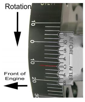
With the engine on the compression stroke on #1 cylinder, set the crankshaft to 10° or 12° before TDC as shown above. Install the distributor so the rotor has just passed the #1 cylinder terminal on the cap as shown above. Make sure you have fuel in the carb, lines and tank. Fire it up!
