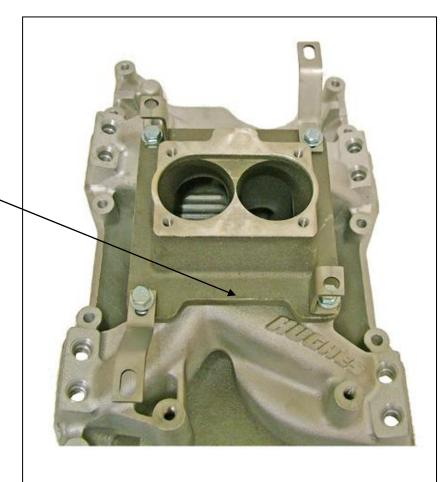
8. With the new FI AirGap on the bench, install your injectors and factory fuel rails on the new manifold. Use some grease or cam break-in lube on the injector O-rings and work the injectors carefully into their bores. DO not damage the O-rings or you will waste a lot of time trying to figure out the engine does not run.
