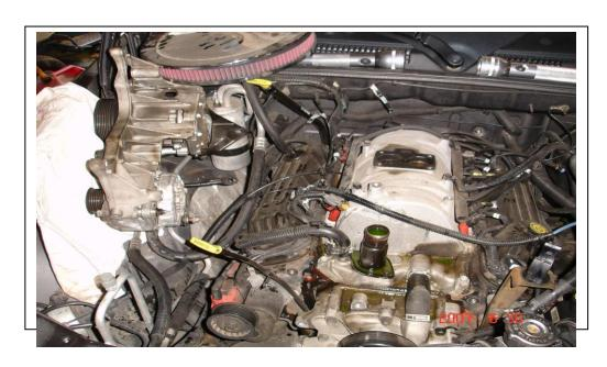
Drain the coolant and disconnect all hoses and wiring harness connectors.
