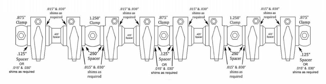
Typical spacer & shim placement for SB Edelbrock RPM head w/ .350" offset rockers.
