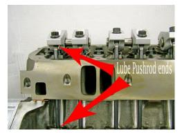
2. Install the rockers. The shafts set in the saddle of the pedestals. The machined flat spots on the shafts go up.
