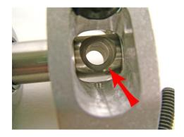
3. Rotate the crankshaft so that the cylinder you are working on is at T.D.C. of the compression stroke (both valves closed). Make sure the pedestals properly align with the rocker shafts before tightening. Torque the hold down screws to 12-14 ft. lbs. Check for pushrod clearance in tunnel. Twist the pedestals back & forth while tightening to make sure the shaft sets correctly in the pedestal.
