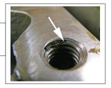
Step 3. Using a sharp chisel and a light tap from a hammer, bend the tail of the thread insert in toward the center of the hole.
