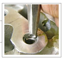
Step 4. Grab the tail of the thread insert with some good heavy-duty needles nose pliers.
