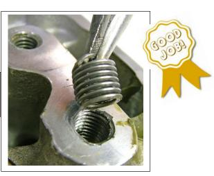
Step 7. It is a good idea to "chase" the threads with a tap. <u>You must use a 7/16"-14 **Helicoil** tap</u> .Normally this can be done with your fingers. No wrenches required—unless you boogered-up the threads with the needle nose pliers.
