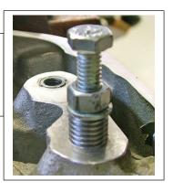
Step 12. Before installing the inserts for the final time clean the threads both in the head and on the insert with brake cleaner or solvent. If you don't, the thread lock will not work very well.
