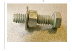
Step 9. Thread on the new insert with the machined side (the pretty side) against the washer.
