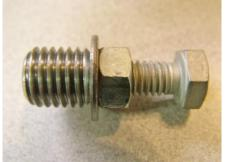
Step 11. The new insert should be thread snugly by hand into the original threaded hole. These inserts are a tight fit.
