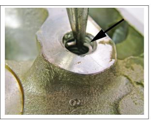
Step 5. Twist the insert counter clockwise (lefty Lucy). The insert is stainless steel so it is stiff and will require some pressure and a tight grip on the pliers.
