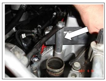
15. All the lines and linkage attach and hook up just like stock. The I.A.T. sensor should be installed in one of the unused 1/4" pipe tapped holes in the side of the plenum.
