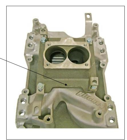
8. Install your Hughes FI AirGap manifold with the intake gaskets and bolts provided. The bolts are a TTY (Torque-to-Yield) type. A diagram showing torque specifications and sequence is on the back page of these instructions.
