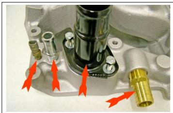
6. Install the thermostat housing and the brass by-pass hose fitting, heater hose fitting, and the coolant temperature sensor.
