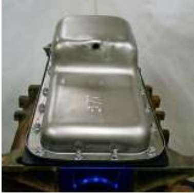
Front and rear view of oil pan. Note the location of the bolts in the front of the pan.
