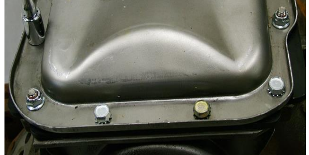
Front and rear view of oil pan. Note the location of the bolts in the front of the pan.
