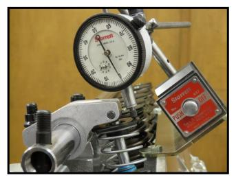
Step 6: Rotate the crankshaft through one complete lift cycle and not the valve lift. Shown here as .610"
