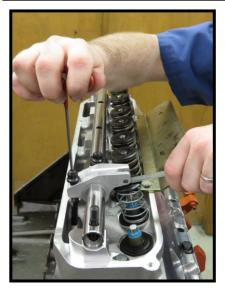
Step 4:Check the wipe pattern at this time. The roller position<br/>with valve closed should start near the position shown,<br/>biased toward the intake side of the head.
