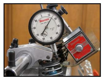
Step 9:If you lost lift when you shortened the pushrod you must go back and lengthen the pushrod 1 turn. ½<br/>turn returns you to the starting length and ½ turn more makes it longer. When lengthening the pushrod,<br/>it will work best if you shorten the rocker adjusting screw first and then lengthen the pushrod to take up<br/>the slack.
