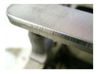
11 Once the proper shim packs and clearances have been determined, rotate the crank and rod assembly by hand and check for proper clearances. The girdles were designed around the 4.00" stroke crankshafts with "H" beam rods. **BUT**, you must check to be sure everything clears! If necessary you can grind off some of the edges; see step 9, clearance, .040" is adequate.
