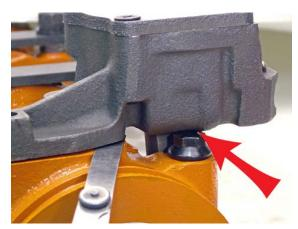
10. Some Magnum oil pans have more draw, angle on their sides, than the "LA" oil pans do. This can cause them to contact the edge of the girdle before seating completely against the block. It may be necessary to slightly grind some material off of the upper outside corner of the girdle plate as shown here. This will not effect the operation of the girdle in any way.
