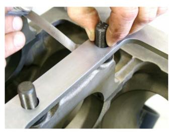
7. Shim each position as required to remove clearance. Double check all positions after shimming. When shimmed properly you will not be able to move or rock the girdle when applying medium finger pressure outboard of the studs.
