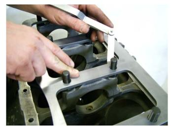
6. To determine the shim requirements you need to lightly hold the stud and girdle as shown here and then use a feeler gauge to determine the thickest blade that can be inserted without moving the girdle. Shims are provided in .002", .005", .008", .010", .015" and .020" thicknesses.
