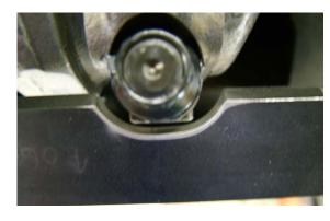
After all the clearances and adjustments are correct, the girdle installation can now be completed. Install a flat washer between the girdle and the nut. Use the provided ARP moly lube on the stud threads and on both sides of the washers. Torque the assembly to 90 ft/lbs. The girdle fits tight enough around the crankshaft to act as a scraper, decreasing windage and increasing power.
