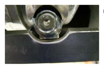
11. Once the proper shim pack clearances and line honing have been completed, rotate the crank and rod assembly by hand and check for proper clearances. The girdles were designed around the 4.00" stroke crankshafts with "H" beam rods. **BUT**, you must check to be sure everything clears! If necessary you can grind off some of the edges (see step #7) for clearance, .040" is adequate.
