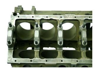
4. Install the main caps in their proper position And install spacers as listed below to start the shimming process.
