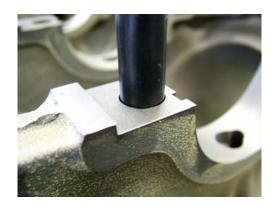
2. The studs should thread in by hand and the shanks should bottom on the block. These studs should only be snug enough (finger tight) to prevent them from spinning out when the nuts are removed.
