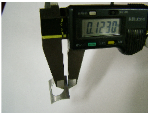
How to measure trimmed shim.
