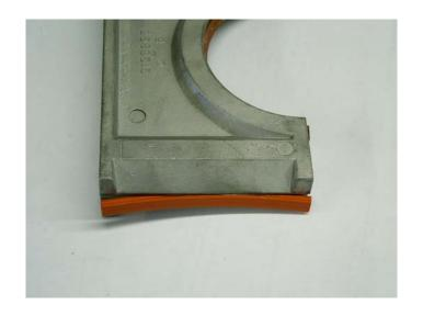
The side seals are the correct lengths – so if you have some sticking up after assembly, <u>do not</u> cut it off – DO IT OVER!
