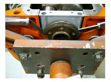
Subtract this total from the wipe length area – example: .498"- .390" = .108" gap. This gap is the distance the rear of the seal hold should be from the front of the flywheel flange when installed. Use feel gauges to set & hold the gap between the flange and the seal holder during final assembly.
