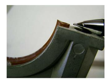
Install the seal in both the block and hold so one end protrudes 1/16" (offset); *more than 1/16*" *can cause leaks*.
