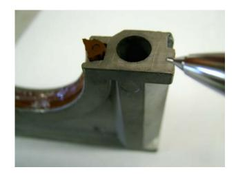
On the bottom ends of the seal hold use a very (very) thin wipe of silicone seal. *More is not better – it can cause leaks!*
