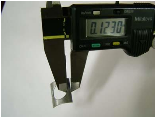
How to measure trimmed shim.
