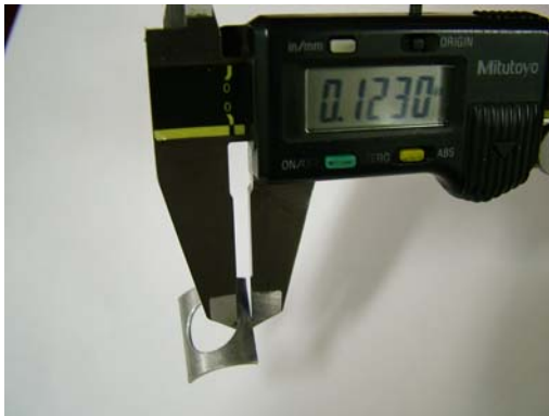
How to measure trimmed shim.
