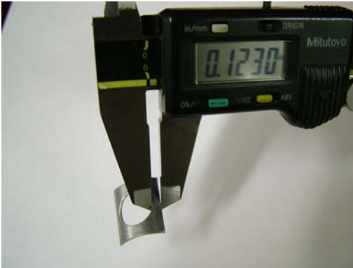
How to measure trimmed shim.
