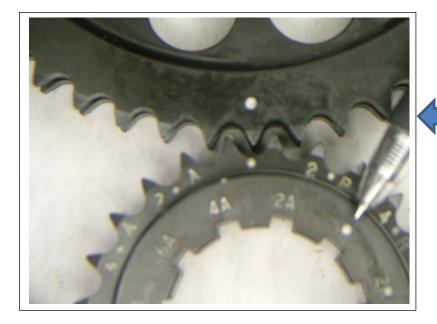
Start the degreeing process with the sprockets in the plain dot-to-dot positions as shown in photo to left. The pen is pointing to the plain dot on the inner keyway. This is the proper location for the crank key.
