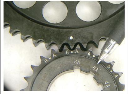
This is the sprockets and cam in the 6ºA (advanced) position and the pen shows where the crank key will be, in the 6A keyway.
