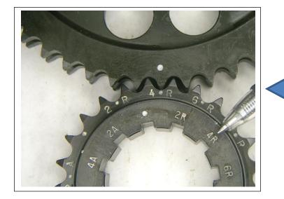
This is an example of the sprockets and cam in the 4°R (retarded) position. Note: The crank key will now be in the 4R keyway position. (The relative position of the crank key will always be in the 2 O'clock position as shown.)
