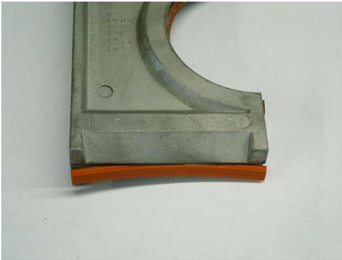
The side seals are the correct lengths – so if you have some sticking up after assembly, do not cut it off – **DO IT OVER!**
